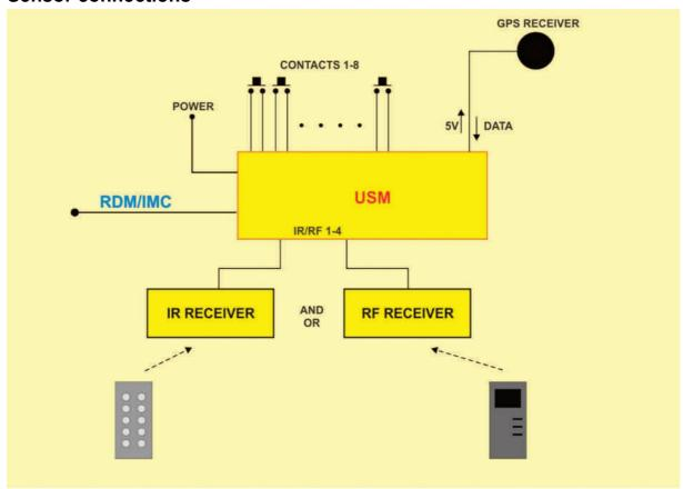
To the RF-IR Receiver input you can connect different type of receiver at same time. It is possible to use four RF, four IR or mixed.
