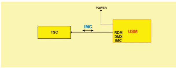
About USM functionality you can read more info also in the manual of TSC controller. For one TSC controller 5 USM module can be connected same time.
